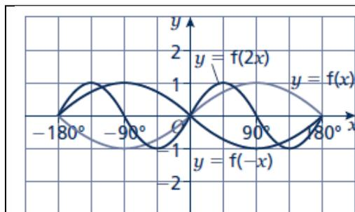
The function  $y = f(2x)$  is a horizontal stretch of  $y = f(x)$  with scale factor  $\frac{1}{2}$  parallel to the  $x$ -axis.
