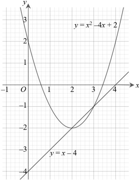
The line and curve intersect at  $x = 3, y = -1$  and  $x = 2, y = -2$
